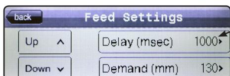
After pressing the On Delay value, a keypad will appear allowing for the number to be changed. The number must be equal to or between 1 and 10,000 milliseconds.
