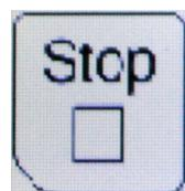
Pressing the stop button will stop the machine and pause the batch counter. The batch counter only runs from the batch counter screen.
