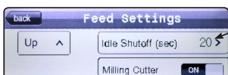
After pressing the idle shutoff value, a keypad will appear allowing for the number to be changed. The number must be equal to or between 20 and 600 seconds.
