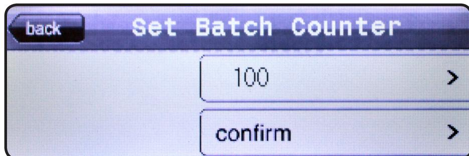
The number in the top box is the current batch counter value. To change this value, press on the number. After pressing on the number, a keypad will appear allowing for the number to be changed. The batch counter can be set equal to or between 1 and 10,000. Once the value has been entered, press the confirm button to set the batch counter value.
