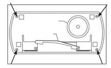
To clear paper jam, remove the plastic paper stop from the bottom of the folder. Turn the large pulley on the left side in either direction while pulling the paper from top or bottom of machine.
