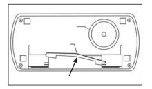
To clean the rubber rollers, spray Martin Yale's Rubber Roller Cleaner and on a clean, lint-free cloth and rub the rollers to wipe them clean. Rotate the rollers by turning the large pulley in either direction. Repeat the process until the rubber and steel rollers are clean and completely dry. Note: Using a cleaner other than Martin Yale's Rubber Roller Cleaner could damage the rollers.
